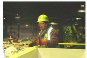
**Naef Recycling** is the other MRF which began processing OCRRA’s curbside material in December, 2002. Naef is a “dual-stream” processing facility. Recyclables are collected and delivered to the facility in a two-compartment truck. At this MRF, all paper is tipped on the floor in one section and all containers are tipped in another section. The material is sorted and baled along two parallel processing lines; one line for paper and one for containers.
