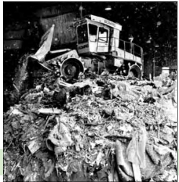
At OCRRA's Ley Creek Transfer station a trash compactor is used to process C&D material. By compacting the material OCRRA minimizes the number of loads it hauls for final disposal which saves fuel and minimizes greenhouse gas emissions.
