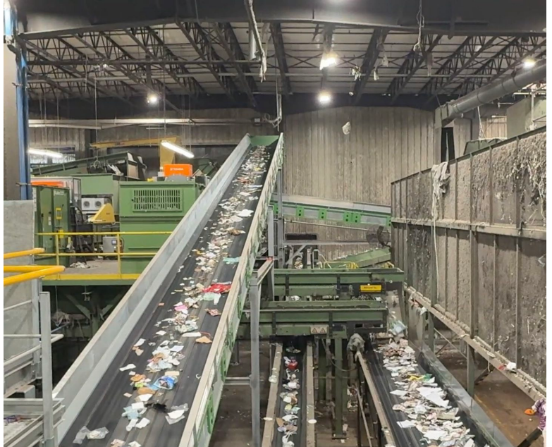
Conveyor lines transporting recyclables at the Syracuse WMRA Materials Recovery Facility (MRF) in Liverpool, NY.
