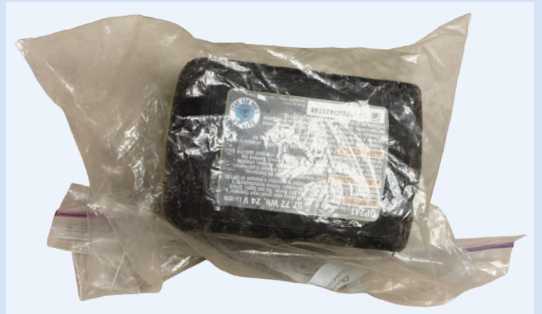
A rechargeable power tool battery, sealed in a zip-top plastic bag to prevent it from falling out.
