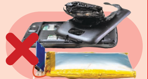
DAMAGED, DEFECTIVE, RECALLED (DDR) BATTERIES
