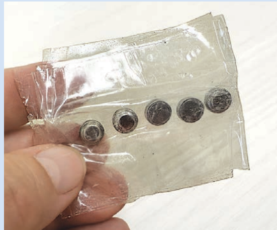
Button batteries separated so they don't touch and terminals are covered by tape.
