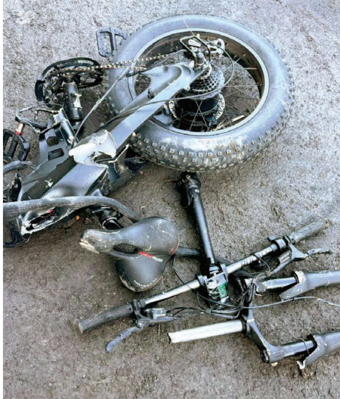
The rechargeable battery on an e-bike ignited after becoming damaged in a scrap metal pile at Rock Cut Road Transfer Station. An OCRRA employee quickly separated and covered the burning battery cells with kitty litter to prevent a larger fire.
