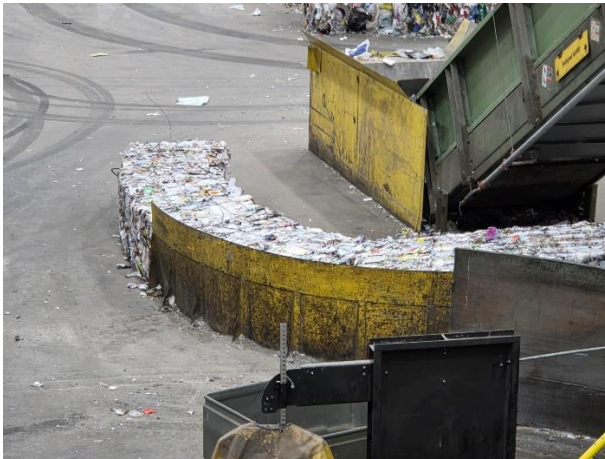
Commodities being baled after running through the conveyor system where optical sorters, screens, and magnets separated them from other materials going to market.
