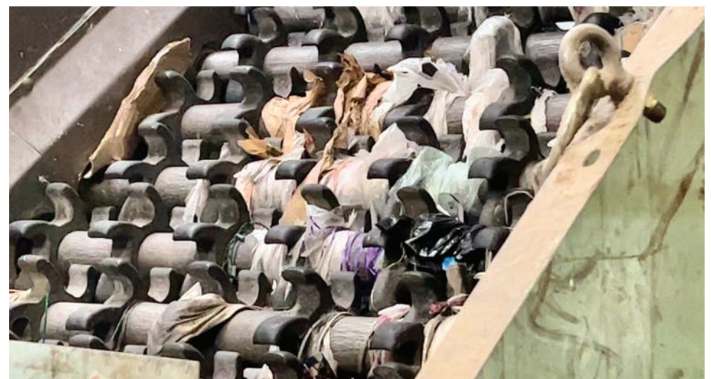
Plastic bags improperly mixed with curbside recyclables wrap around rollers on equipment used to sort different types of recyclables.
