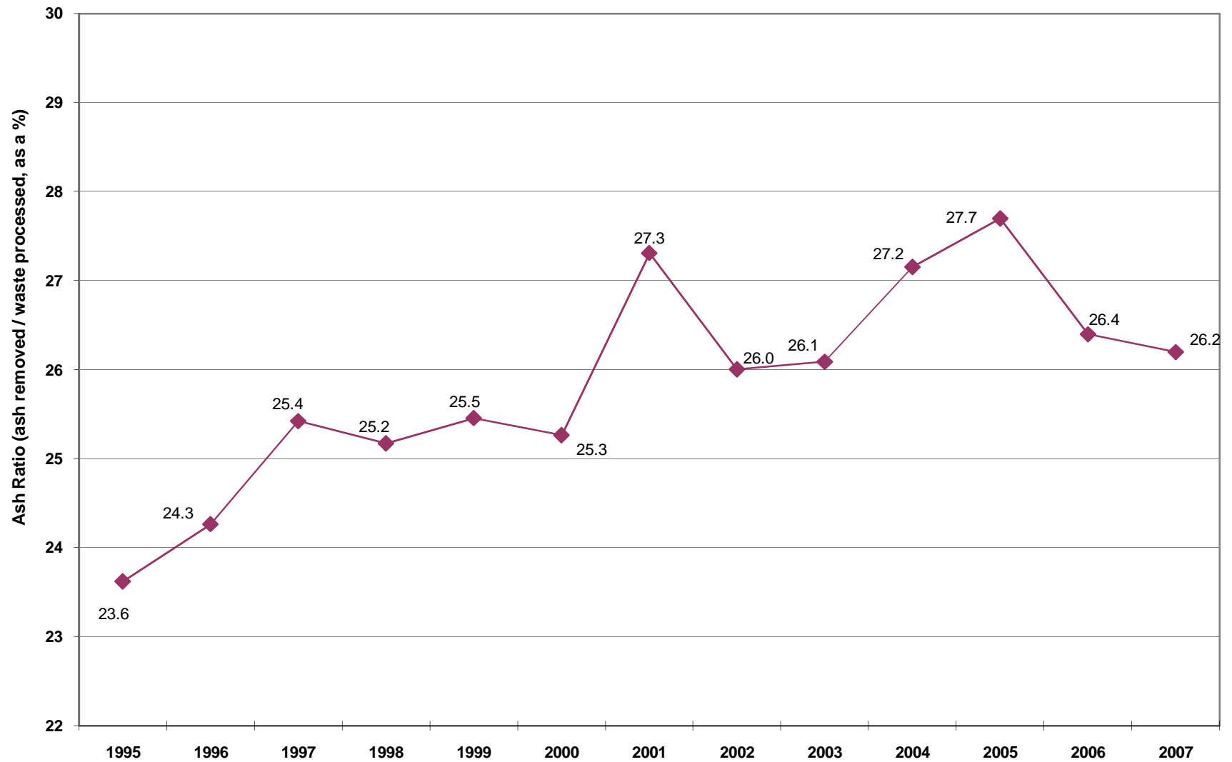
Figure 5. Annual Average Ash Ratio as Percent of Throughput Onondaga County Resource Recovery Facility
