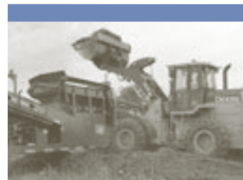
This trommel screens out all particles larger than a half inch thus producing top quality compost. OCRRA compost customers have come to expect top shelf soil supplements from our two locations.
