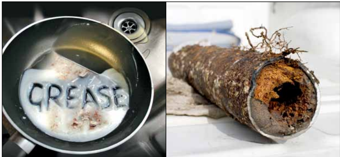
Fats, oils and grease (FOG) from cooking clogs pipes (like the one above, right) and can inflict costly damage to property as well as the environment. Prevent sewer backups by throwing FOG in the trash instead of down the drain. Or, recycle it for free at the Metropolitan Wastewater Treatment Plant on Hiawatha Boulevard in Syracuse.
